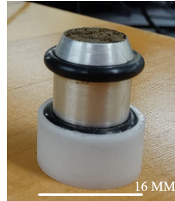
Figure 20: An image of the sample cylinders with beveled edges containing a sample of collected soil.
